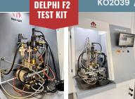
Delphi Euro-6 F2e Series Pumping & Non-pumping Injector Test Kit. Ko2O39 has a high-pressure rail that can control pressure up to 2200 bar.
