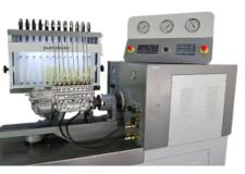
Powerful Drive System PT2012 B has a Special design 20 HP AC motor providing high torque at low
