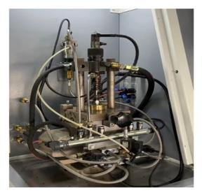
KO2039 has a high-pressure rail that can control pressure up to 2200 bar.
