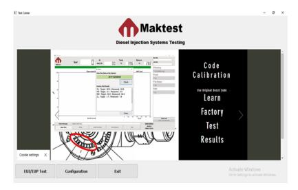
UTS1004 user interface provides all the necessary data on the test screen readily available for the user to decide the condition of the injector. The software allows the use to create different test plans.
