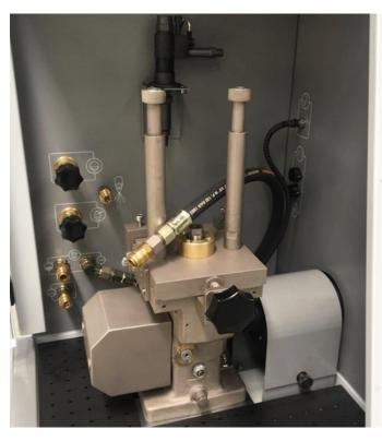
Patented Cam Box; stroke set between 10 & 18 mm.
