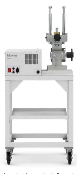
Electronic Drive Module drives the injectors electrically, results are read from the host test bench and manually entered into the computer software for results display and analysis. The control box may be on a desktop.
