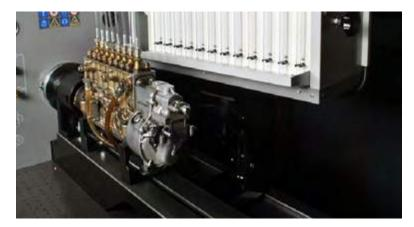
The ø110 mm coupling ensures your safety with its durable and strong design and provides reliable testing of the new technology high- pressure output fuel injection pumps.
